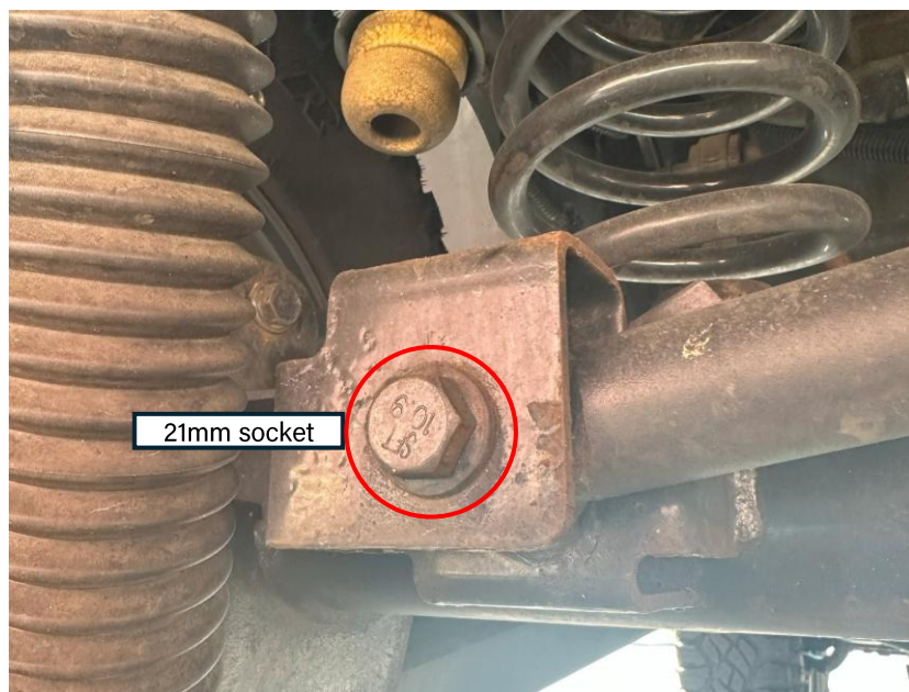
JK axle-side rear track bar bolt to be removed (OEM mount)
