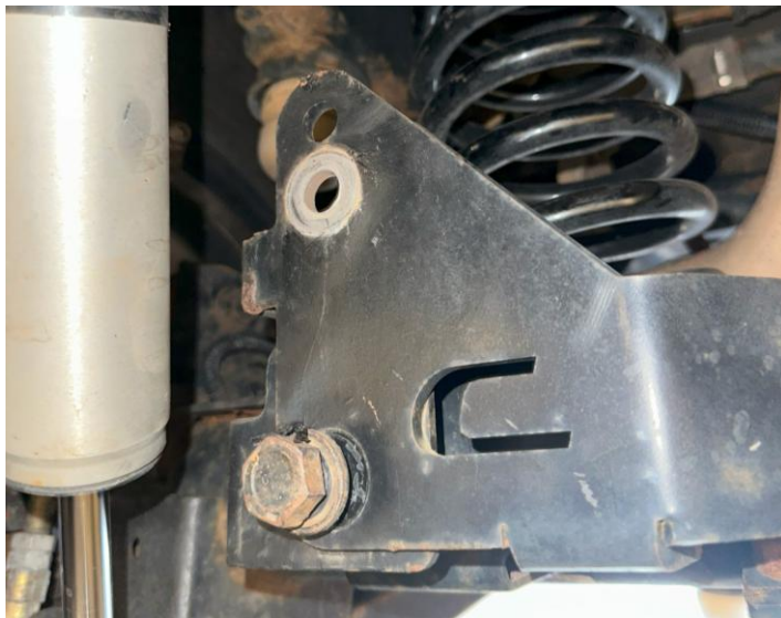
JK adjustable rear track bar bolt installed hand-tight (axle-end)
