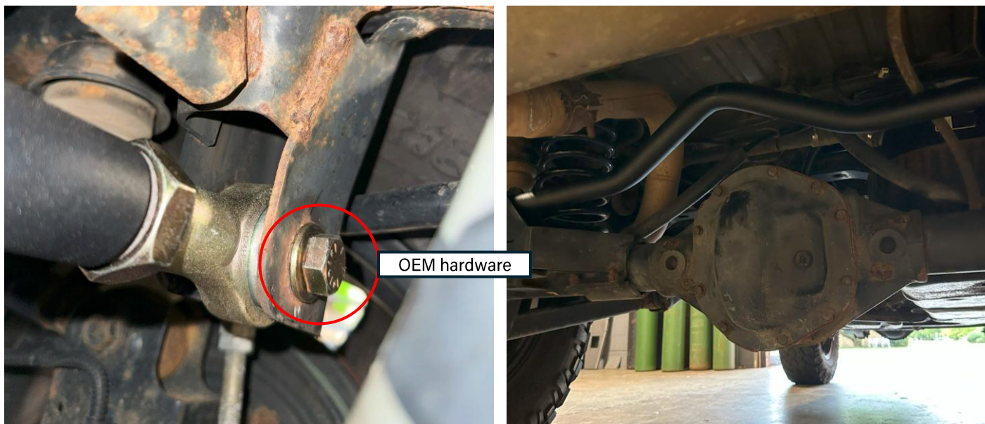
JK rear adjustable track bar installed at frame end with the bend in the bar providing clearance for the differential
