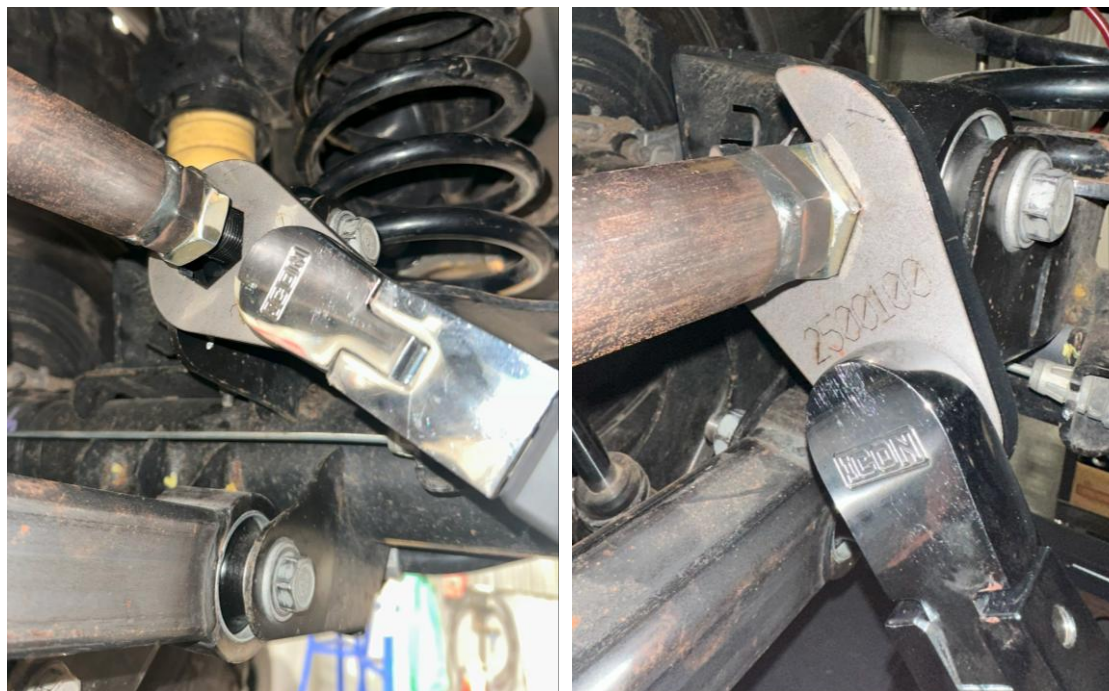
Figure 2: Crow's Foot Wrench slipped over threaded shank and onto jam nut
