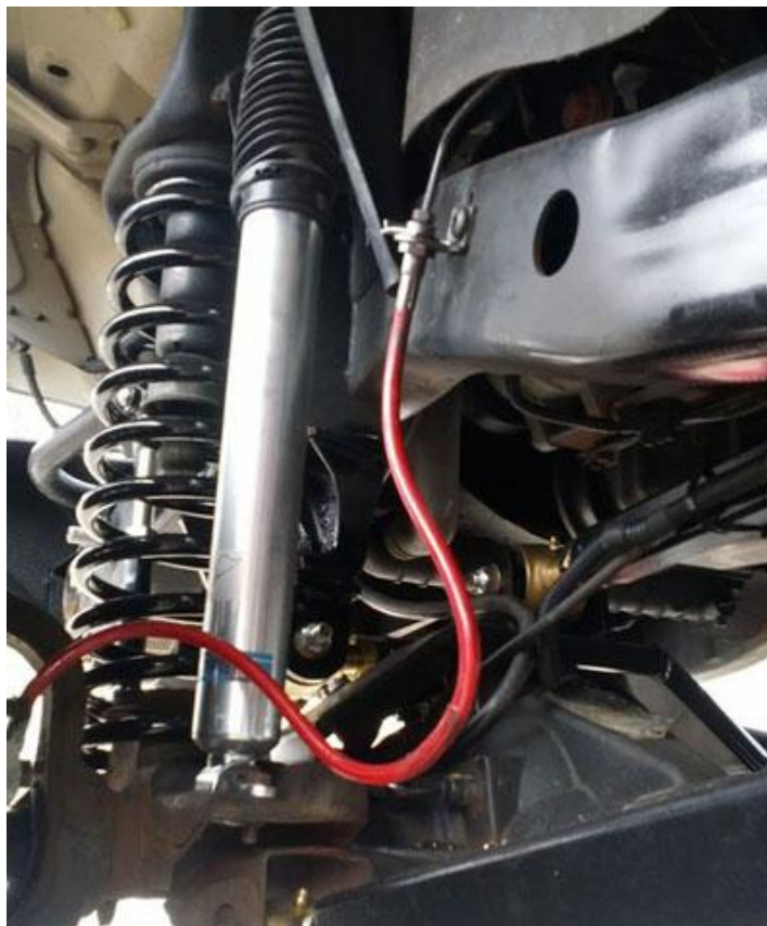
Frame-side brake bracket with new brake line installed
