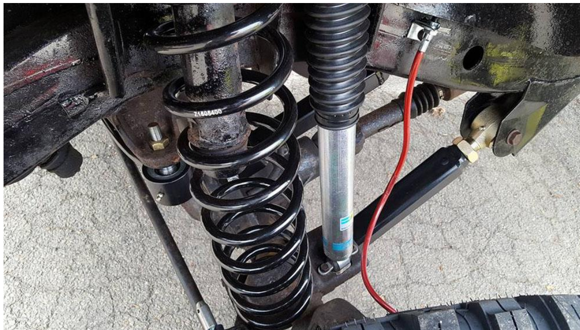
Frame-side brake bracket with new brake line installed
